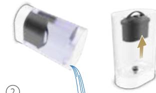
② Empty water tank and remove water filter.
